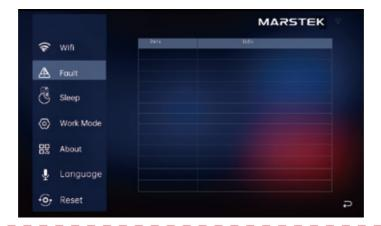
Touch Sleep button to set 10 min/20 min/30 min or never. If M5000 is standby(no grid, PV, or load connection) via battery module only, the system will automatically trips when the set hibernation time ends(breaker will turn off). if connect load, the system will not sleep.
