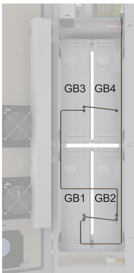
Figure 4.14 Battery communication cables
