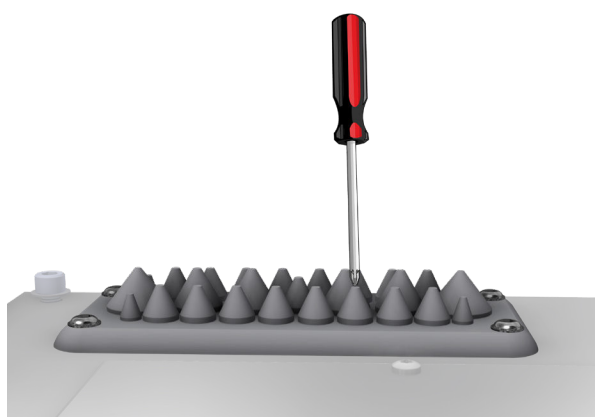
Figure 4.2 Cable glands preparation
