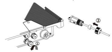
Insert the cable into the corresponding communication connector in the order of the arrow, tighten the sleeve and the forcing head screw at the tail.
