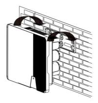
4. Check both sides of the outer fin of the inverter to ensure that it is securely in place.
