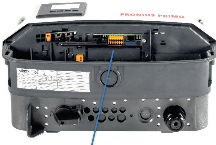
Figure 3: 16-pole plug on SnapINverters (Primo, Galvo, Symo, Eco). Pin IO 0-3 and GND (-) to be used to control the external relay.
